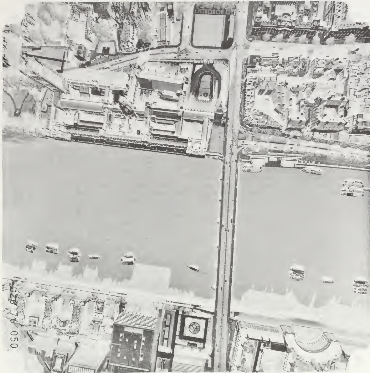
Figure 13: Aerial photograph of (top left) the Houses of Parliament and (right of centre) Westminster Bridge, London. Because they are viewed from a finite altitude, the tops of buildings appear farther from the centre of the picture than the foundations.
